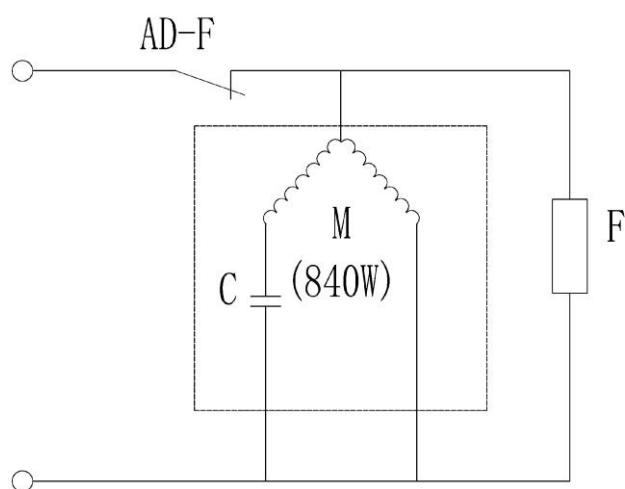
AD-F: pressure switch    C: electric capacity
