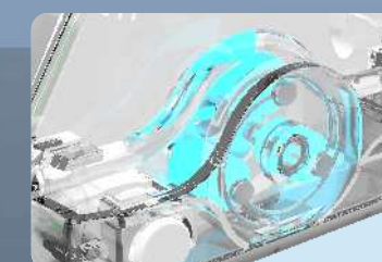
Silent, waterproof peristaltic pump
