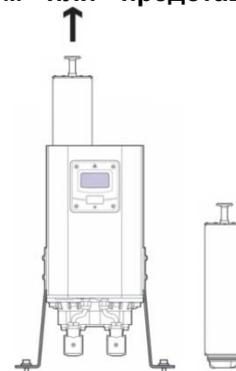
Fig.14-B: Dryer cartridge
